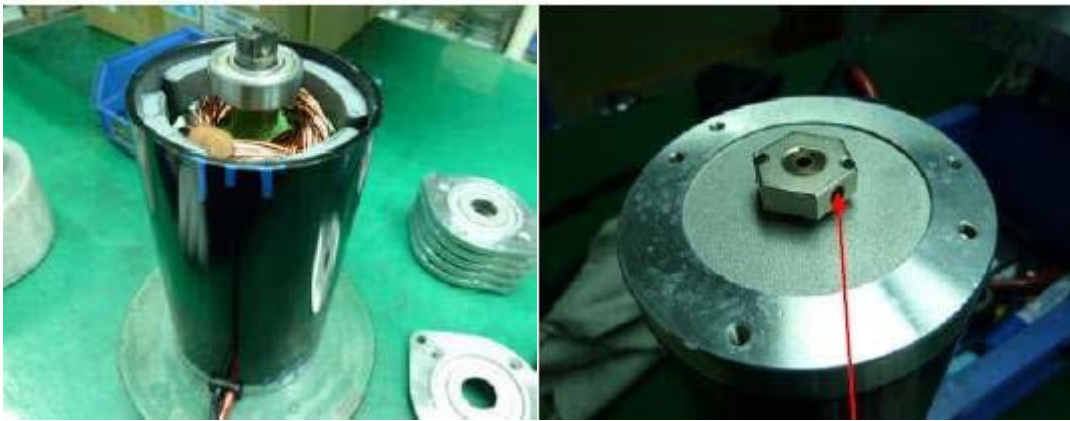
Step 10: Put the outer tube back and put the front bracket back and tighten the hexagon nut.
