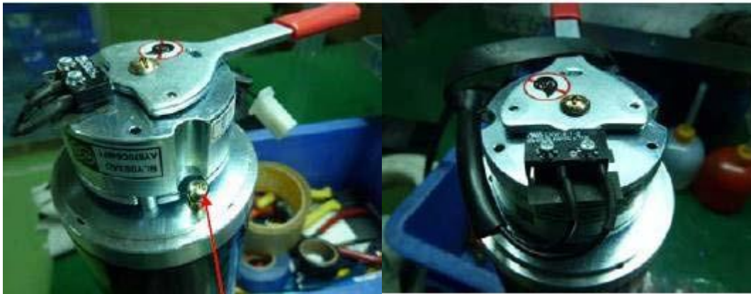
Step 11: Reinstall the brake device and put the dust-proof cover back. Done !
