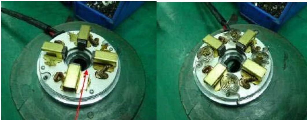
Step 8: Insert the waved-shape pad into the bearing hole. Insert 4 units of brush springs
