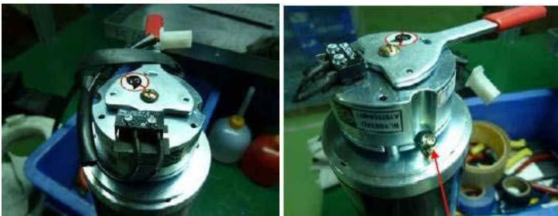
Step 2: Separate the brake plug from the connector and then witch the brake lever to the DRIVE. Loosen the screws properly
