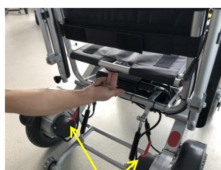
Push or pull two red electromagnetic brake switch
